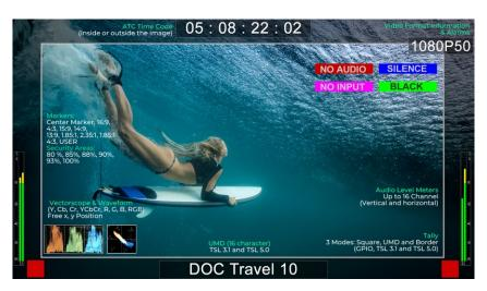
Pluma monitors have all professional features and adjustments as UMD and Tally, Blue Only, Aspect Ratio Selection, Markers, Real time color Waveform and Vectorscope per input (SDI 1 and SDI2), 16 Channel Audio Level Meters, Alarms, Timecodes, backlight and color temperature adjustment (5600K, 6500K, 9300K, and RGB Gain and Bias adjustment), and more.
