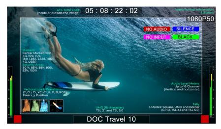
These monitors have all professional features and adjustments as UMD and Tally, Blue Only, Aspect Ratio Selection, Markers, Real time color Waveform and Vectorscope per input (SDI 1 and SDI2), 16 Channel Audio Level Meters, Alarms, Timecodes, backlight and color temperature adjustment (5600K, 6500K, 9300K, and RGB Gain and Bias adjustment), and more.
